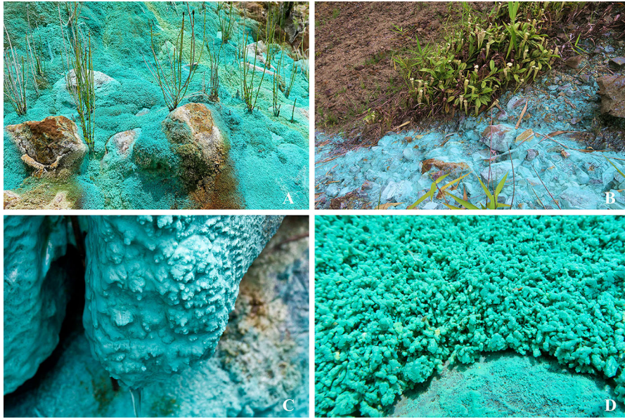
Fig. 3 Formation of the mineral brochantite on boulders overflowed with acidic Cu-rich mine water
