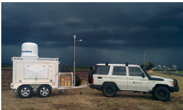
FIG. 3. Photograph of the mobile X-band dual-polarized radar deployed with mobile weather station at Gatton, SEQ (see Fig. 1), on 26 Nov 2014.
