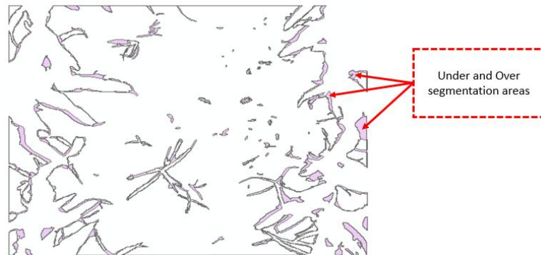
Figure 6-27: Symmetrical Difference Map showing areas of over and under-segmentation (Symmetrical Difference Result)
