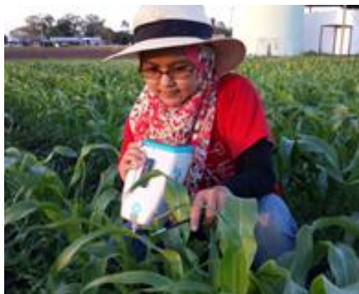
Figure 3-11 Collecting spectral signatures using the FieldSpec® HandHeld 2™ Spectroradiometer with fibre optic attached.
