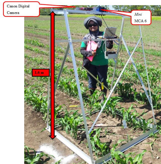
Figure 3-15 Taking the quadrant image using a jig
