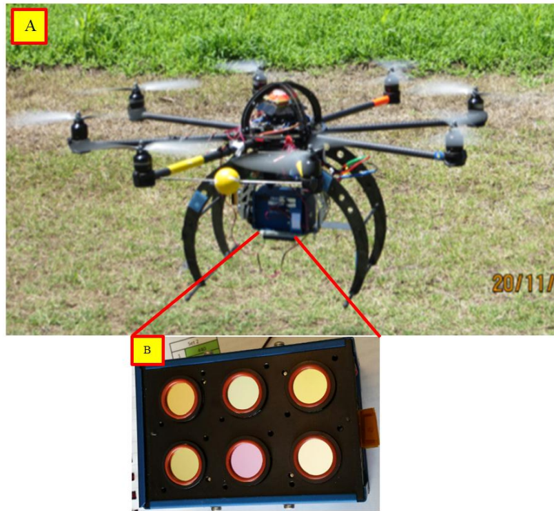
Figure 3-13 Mini Multi Channel Array (MCA6) camera attached to the Mikrokopter JR11X (A) and MCA 6 in close up without cover (B)
