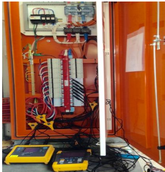
Figure 5.8. Measurement Test Setup for Harmonic Analysis.
