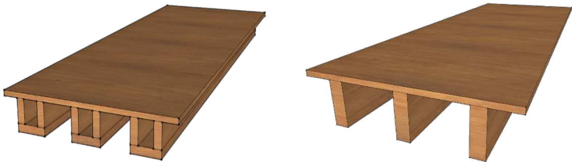
Figure 1 Illustration of composite box-shaped LVL floor (left) and composite T-shaped LVL floor (right)
