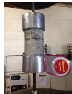
Figure 12 A sample in direct tensile test
