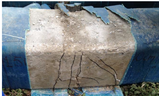
Figure 13 Autopsy of ImpA1, after the second impact
