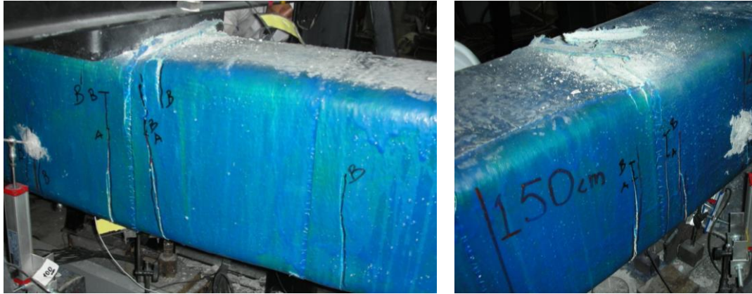
a. Vertical cracks at the loading region b. Rupture of the Aramid fibers at the top surface Figure 11 Damage of ImpA1, after the second impact
