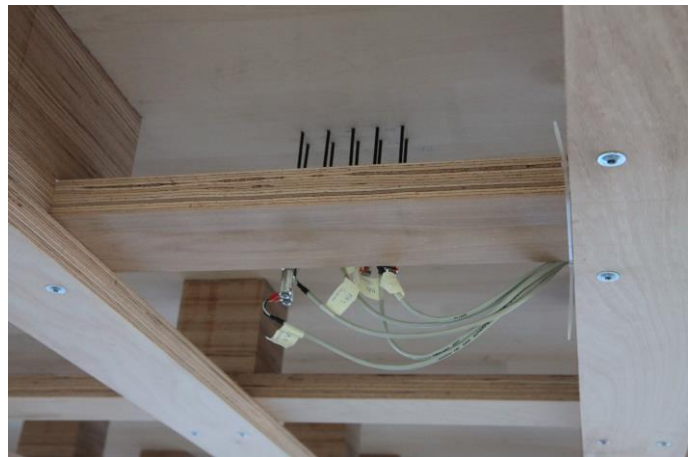
Figure 4 Moisture content measurement inside the timber a) Insulated steel needles inside a timber column b) Insulated steel needles inside the beech CLT plate at 5 different depths
