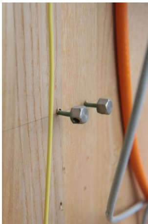
Figure 4 Moisture content measurement inside the timber a) Insulated steel needles inside a timber column b) Insulated steel needles inside the beech CLT plate at 5 different depths
