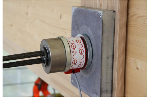
Figure 3 a) Joint between the column and the beams b) Installation of a load cell (tendon anchorage point)
