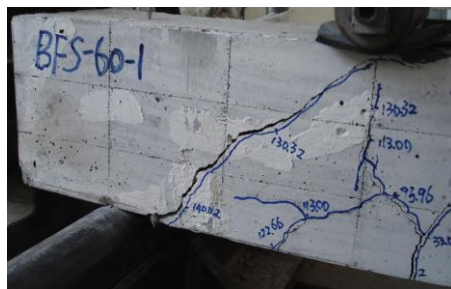
(a) Shear-compression failure (BFS-60-1)
