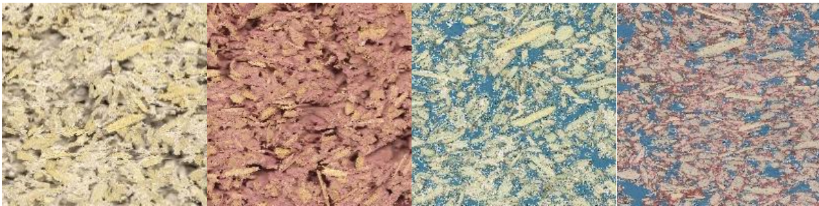
Figure 1 Comparison freshly cut hemp-lime, freshly cut pigmented hemp-lime, resin encased hemp-lime, and pigmented & resin encased hemp-lime
