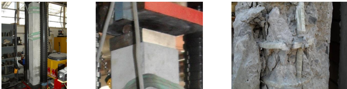
Figure 1 Left: Column in Amsler Machine. Centre: Steel Plate. Right: Ruptured GFRP Bar and Tie.
