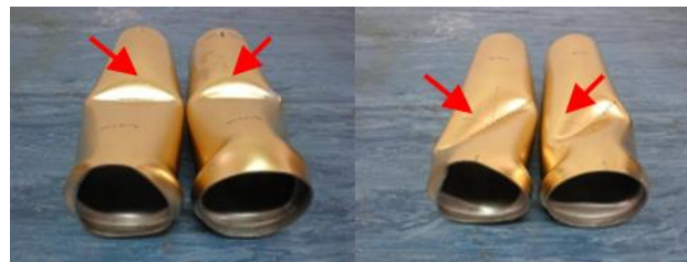
Figure 2 Failure mode of the tube specimens with different dent shapes under compression.
