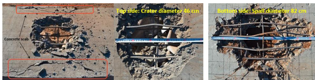
Figure 5 NRC slab under 1 kg TNT contact explosion
