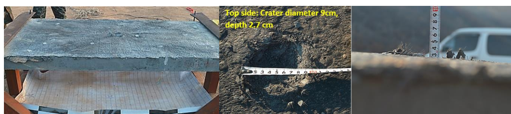
Figure 6 UHPC slab under 0.1 kg TNT contact explosion
