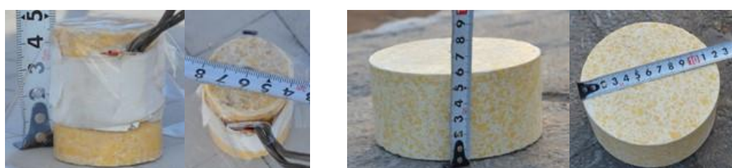
(a) 0.1 kg cylindrical TNT explosive
