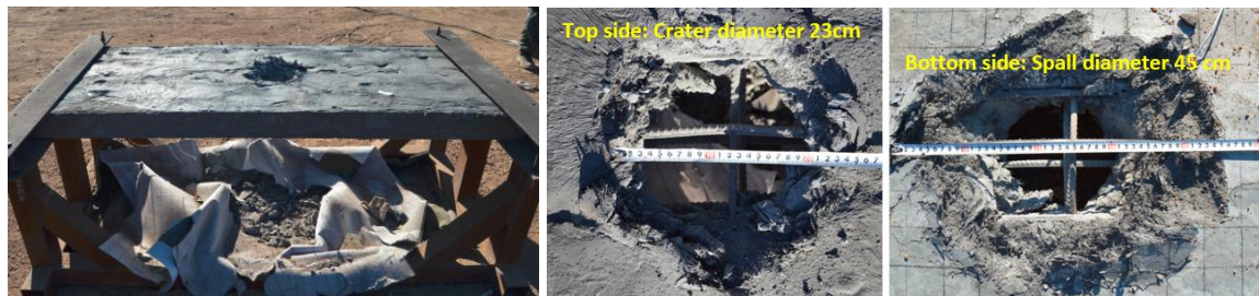
Figure 7 UHPC slab under 1 kg TNT contact explosion
