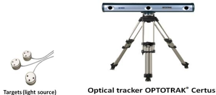
Figure 2 Optical sensing system; (a) target (light source); (b) optical tracker;
