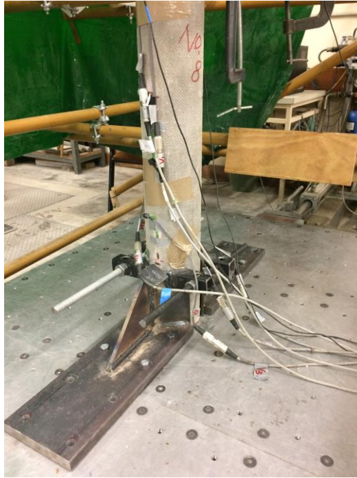
Figure 4 A composite column fixed to shake table with steel supports
