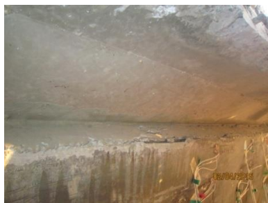
(a) Stripping damage of SPCCS-S-1
