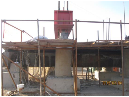
Figure 3 Loading device of shear resistance test
