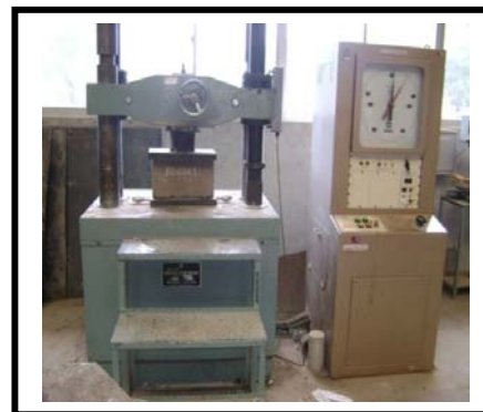
(b) testing of CEB in compression
