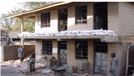
(b) Rammed earth building under test loads
