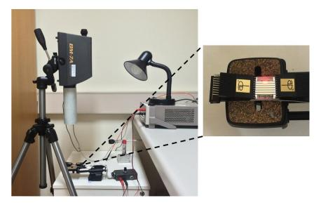
Figure 2.7 Two photographs showing the experimental set-up for OLED testing utilised at the CSIRO test facility.
