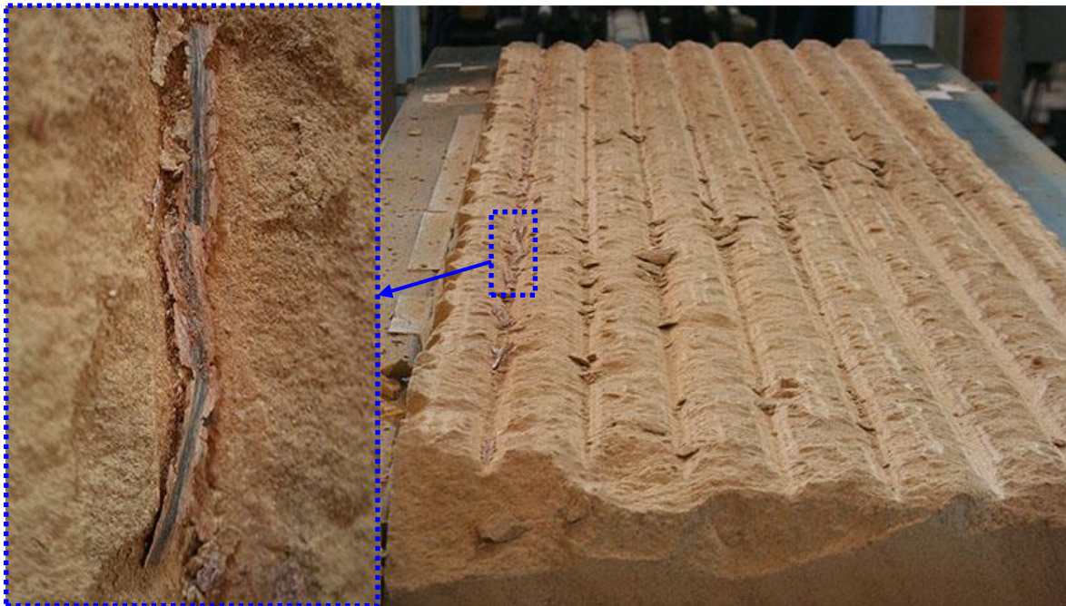
Figure 5.23 Reddish and black discontinuous banding chips was found in the cutting grooves when the cutting temperature reached 1100 °C ( v = 2.5 m/s, d = 10 mm, s = 50 mm)
