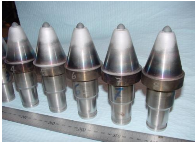
Figure 3.8 TSDC tipped SMART*CUT picks
