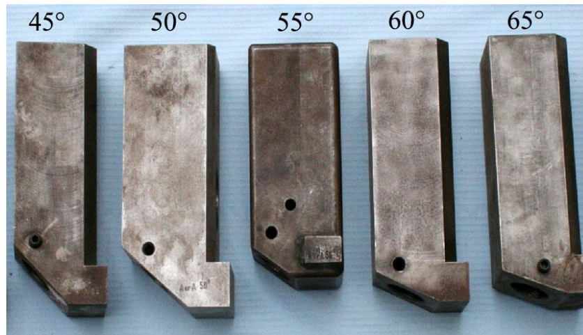
Figure 3.9 Tool holders with different attack angles (45, 50, 55, 60 and 65 degree respectively)
