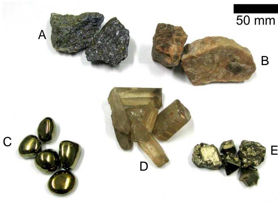
Figure 3-7 – Unprocessed mineral specimens: molybdenite (A), feldspar (B), chalcopyrite (C), quartz (D) and pyrite (E)
