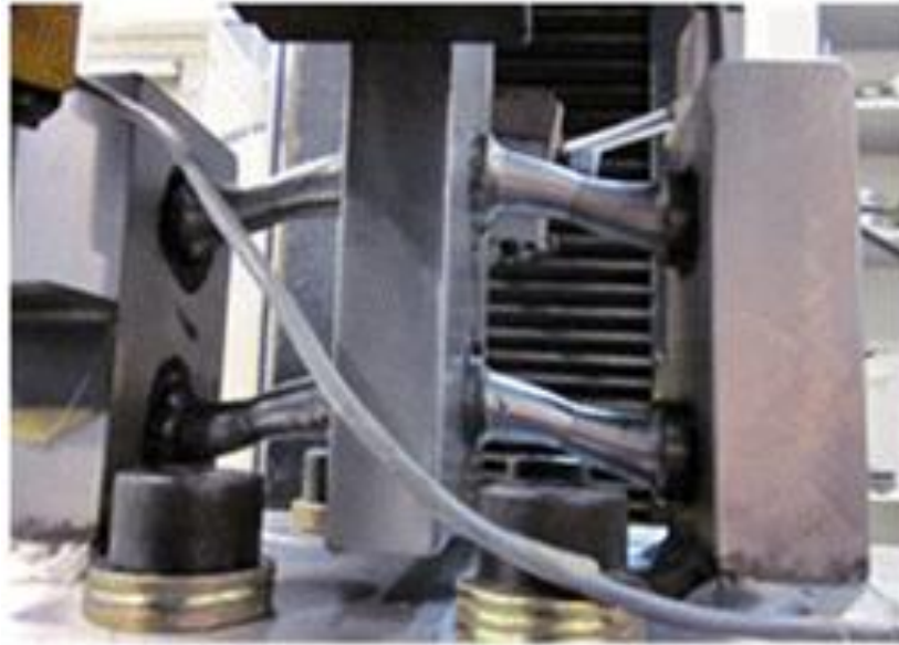
Figure 3.26 Setup for WHP component tests
