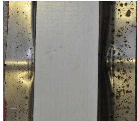
d) Impactor deformation top view, hybrid sample
