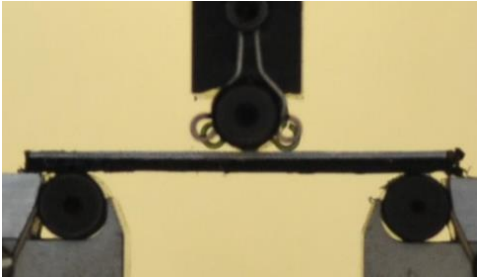
Figure 4-7: Quasi-static three-point bend set up with composite face down (S/C) – sample length 60 mm, span 40 mm, width 15 mm
