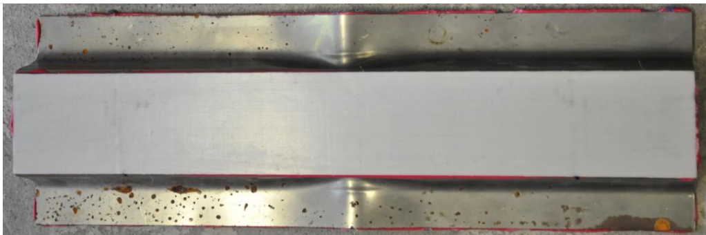
b) Tested sample with composite reinforcement, top-hat side down scenario
