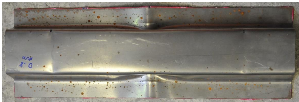
a) 0.8 mm pure steel sample
