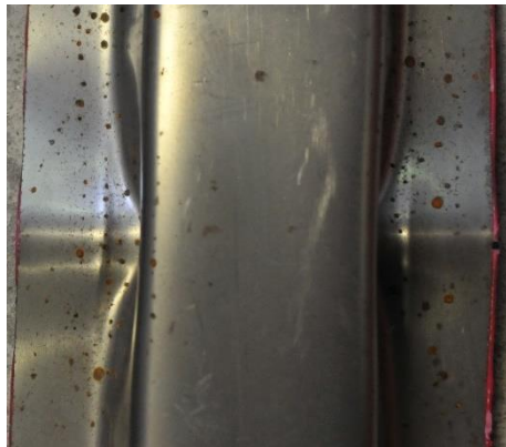
c) Impactor deformation top view, pure steel sample
