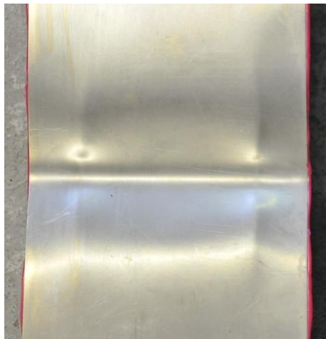
a) Impactor deformation on backplate of 0.8 mm pure steel sample
