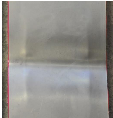
b) Impactor deformation on backplate of 0.8 mm hybrid sample
