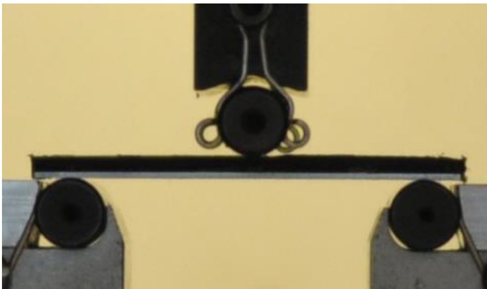
Figure 4-8: Quasi-static three-point bend set up with steel face down (C/S) – sample length 60 mm, span 40 mm, width 15 mm
