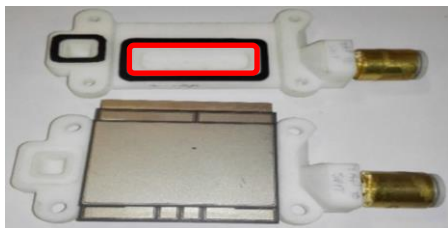
Fig. 3 – The liquid cooler applied to the HBS.
