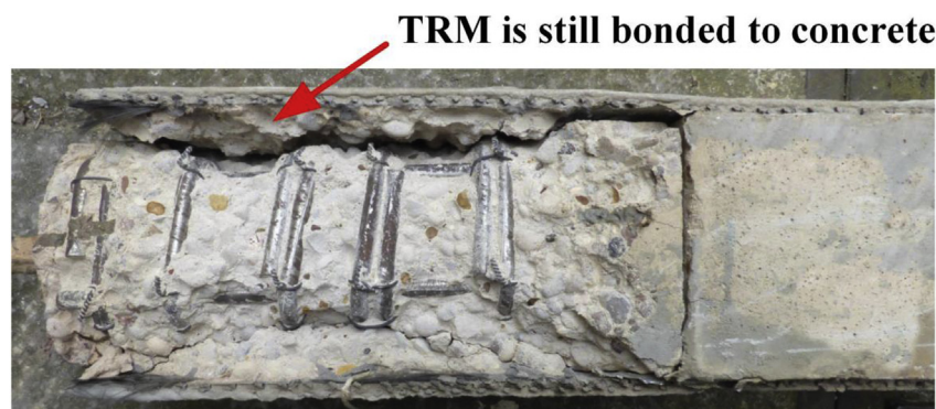
Fig. 17. Exploded specimen heated up to 550 °C.
