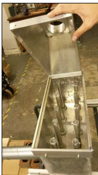
Figure 2 (a) Internal view of reactor showing perforated diffuser pipe allocation
