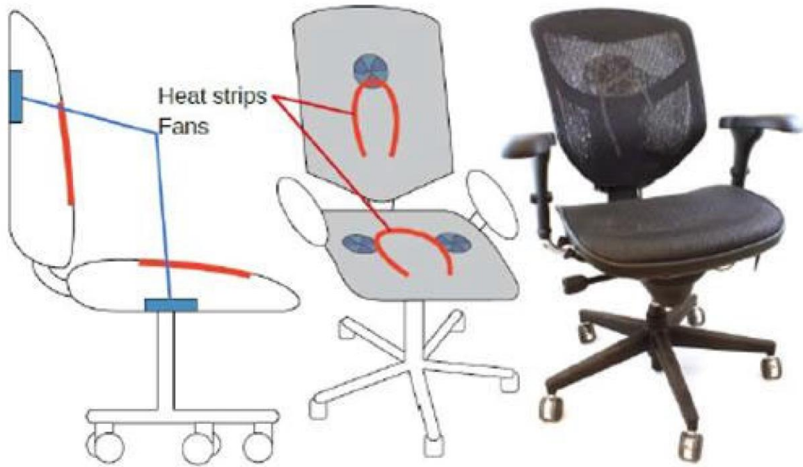
Figure 1. The Personal Comfort System Chair, UC Berkeley [38]
