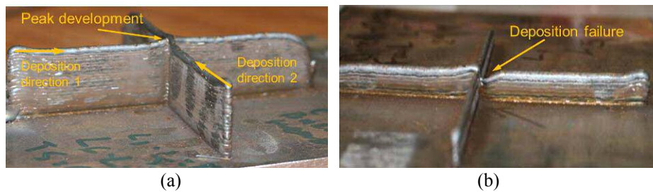
Figure 6 Undesirable features of crossing structure: (a) Peak development; (b) deposition failure (see online version for colours)
