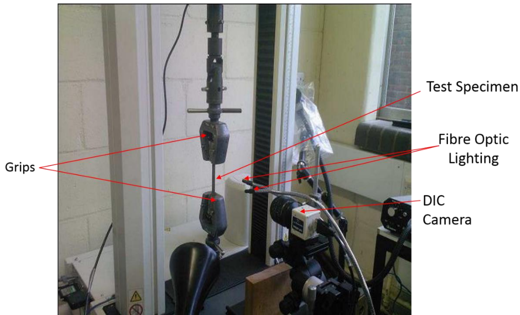
Figure 2-21: Optical image of 2D DIC acquisition system.
