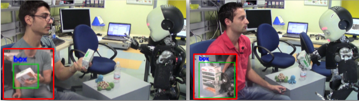
Figure 2. The Human-Robot Interaction setting. The iCub’s motion detector (left) and forward kinematics (right) both provide a reasonably good estimation of the object position within the image.
