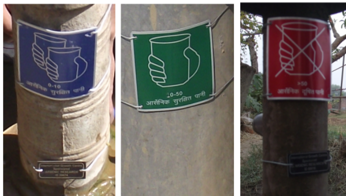
Figure 2 Metal placards with test results attached to pumphead
