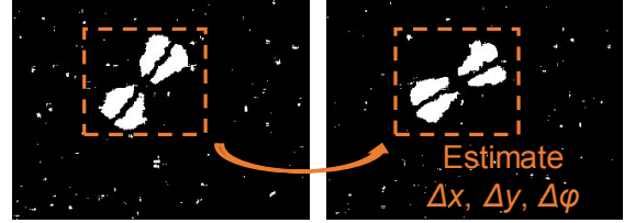
Figure 6. Consecutive “difference” frames. A value of ‘1’ indicates “test frame” pixel values that have non-overlapping 95% confidence intervals in consecutive frames.
