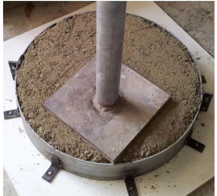
Figure 3. Initial manual compaction of specimen.
