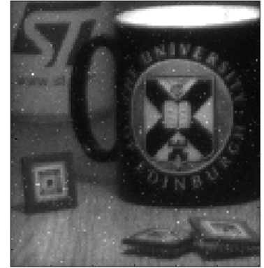
Fig. 3. Single shot grayscale intensity image with no post processing. White dots are high DCR pixels.
