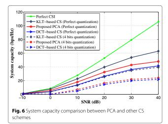
the BS can acquire perfect CSI with neither recovery distortion nor quantization error. As illustrated in Fig. 6, the best system capacity can be achieved only when the BS acquires perfect CSI. Meanwhile, the proposed scheme outperforms the existing DCT-based CS scheme whether there is quantization error resulting from lowdimensional CSI or not. But, it performs a little poorer than the KLT-based CS scheme.
