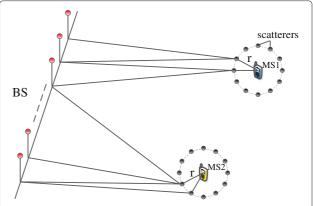
**Fig. 1** Illustration of the one-ring model with Q scatterers uniformly distributed on a circle of radius r
