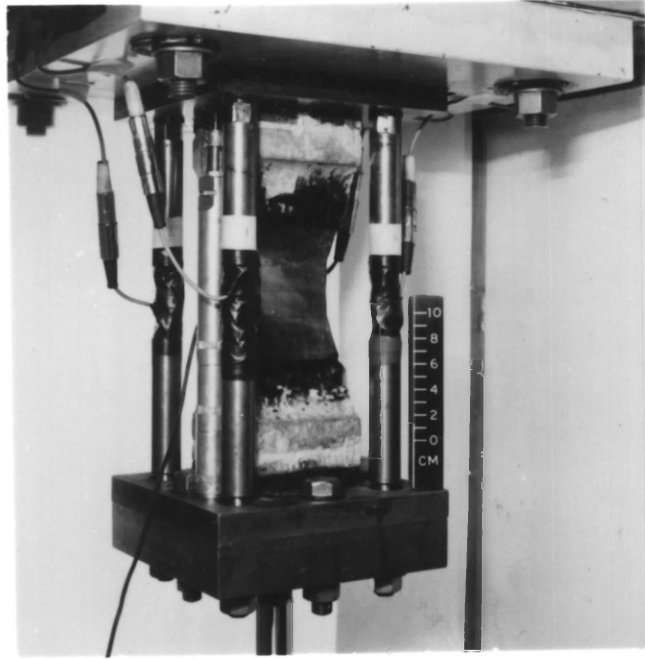
Fig. 4.2 Specimen mounted in testing machine
