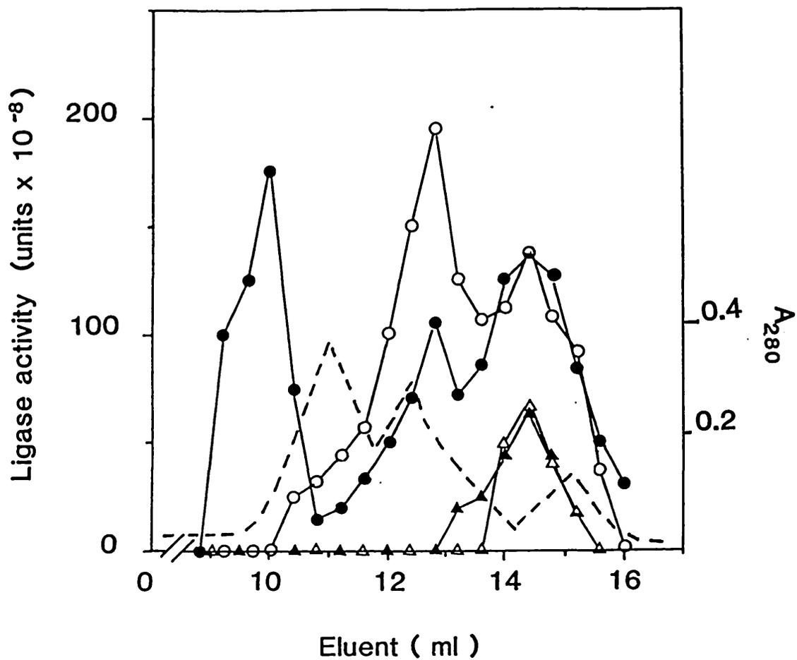
Fig. 4.15 DNA ligase activities in the cell line 46BR, containing a dimeric form of DNA ligase I and in Cockayne's syndrome cell line, GM1712. FPLC elution profiles and symbols are the same as in Fig. 4.3.
