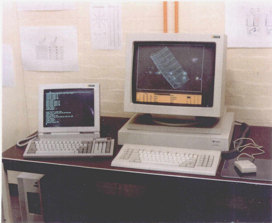
Plate 15 : The SUN 3/60 Workstation onto Which The Blade Modeller and Integrated Inspection System were Transported
