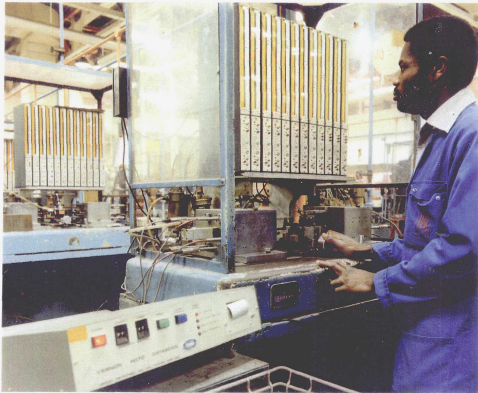
Plate 7 : Gauging of Blade Surfaces By Drop Gauge Fixturing
