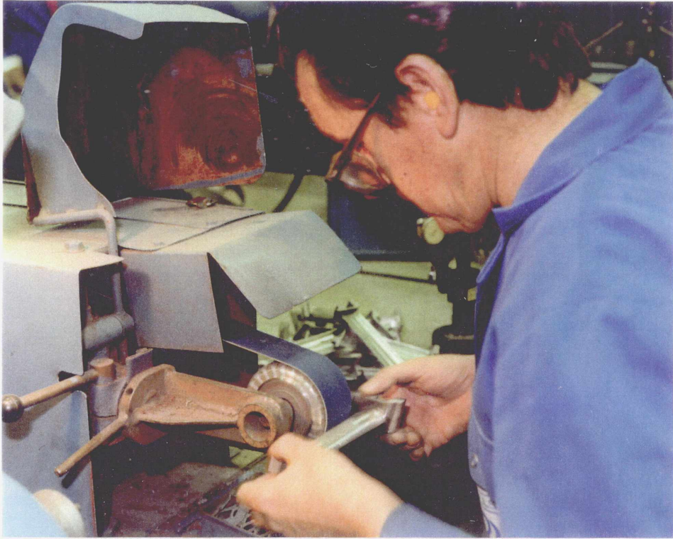
Plate 6 : Manual Grinding of Casting Surfaces
