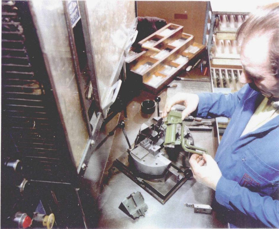
Plate 2 : Blade Wax Pattern Injection Around a Ceramic Core
