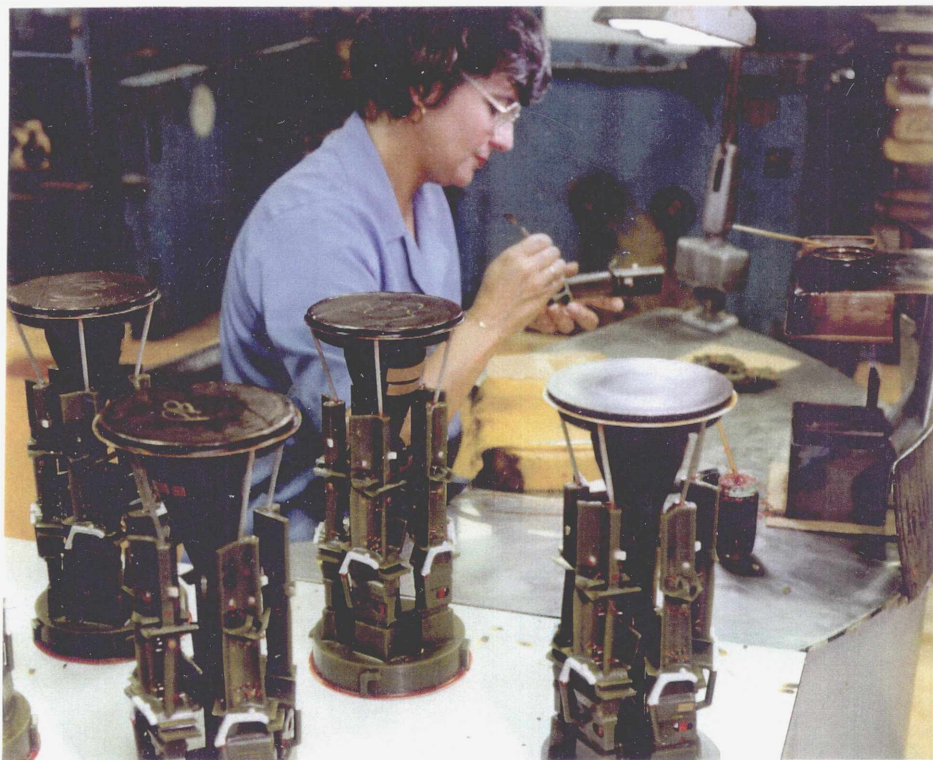
Plate 3 : Construction of the Blade Casting Runner/Riser System
