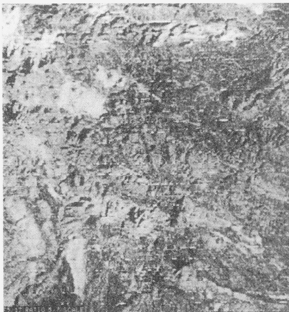
(a) Original TM 5/7 ratio. Note the periodic and isolated noise
