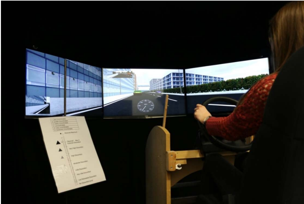
Figure 2: Driving simulator configuration
