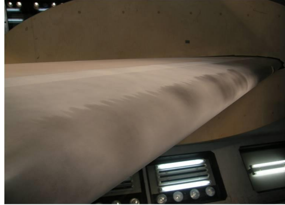
Figure 10 Transition front visualised by china clay technique
