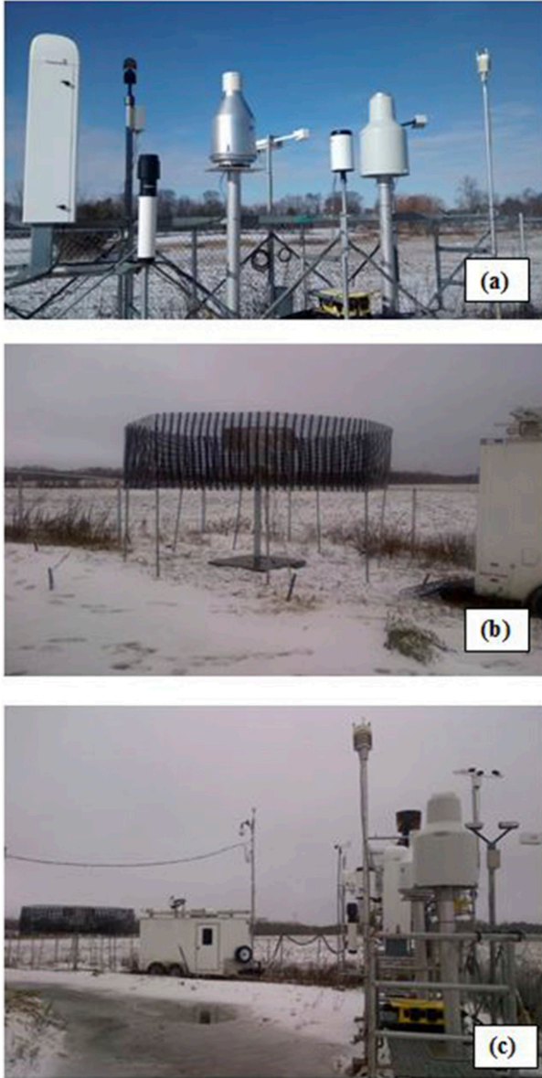
FIG. 6-3. Various precipitation sensors at the PUMS site near Toronto, Ontario, Canada. (a) The Geonor, Pluvio, Yonge tipping-bucket, capacitor sensor, and WXT52. (b) A double-fenced reference system with Pluvio sensor (scaled down to 1.5 times), similar to the DFIR reference platform. (c) Entire project area (PUMS site) in Oshawa.
