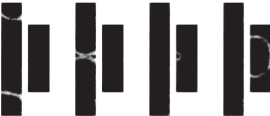
Figure 2. Four photographs of a chemical coincidence detector. Each photo has two sections of active substrate, the left-most acting as inputs, the right-most as output. The waves are inputted (from the top and bottom), and as they collide, the activator concentration between them rises higher than if only one wave was present. This results in the activator diffusing farther into the gap between input and output section, producing a wave on the output section (Reprinted with permission from [18]. Copyright (2003) American Chemical Society).
