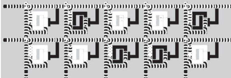
Figure 19. Two columns (rotated) are successfully trained with distinct patterns, without interference or crosstalk between the patterns. First pattern (bottom) is the binary value of 25 (11001); second pattern (top) is the binary value of 21 (10110).
