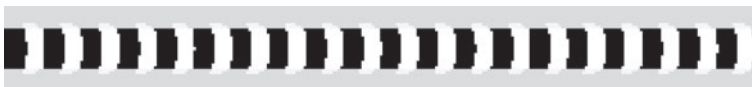
Figure 5. Example time-lapse output from the simulator. The activator concentration is thresholded at u = 0.04 every 1000 simulated time-steps, and marked as white. The illuminated (passive) regions of reactor (high \phi ) are signified by grey background, and non-illuminated (active) regions of reactor (low \phi ) are black.
