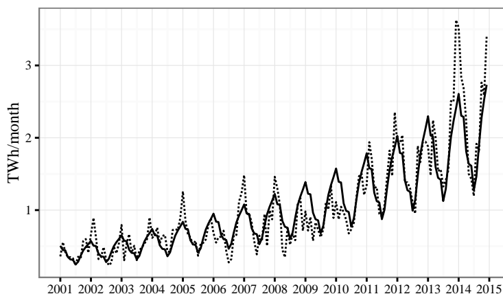
Figure 6: The figure shows the historical mean monthly wind output (dotted line) and the fitted wind output (solid line) from a regression of wind generation on monthly dummies and time trend. Units are in TWh/month. Data from years 2001–2014.
