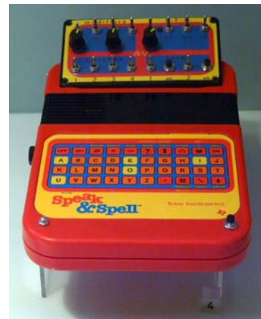
Figure 3 – A Circuit-Bent Speak & Spell, as exhibited at the London Science Museum. Switches, buttons and potentiometers have been added to the device, controlling the modifications made to its circuits (Image copyright Loz Pycock, CC BY-SA).
