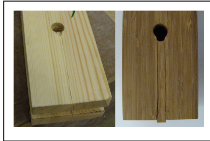
Figure 6: Fracture in timber (left) and engineered bamboo (right).
