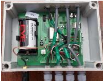
Figure 1. Wireless strain sensor node developed in CSIC
