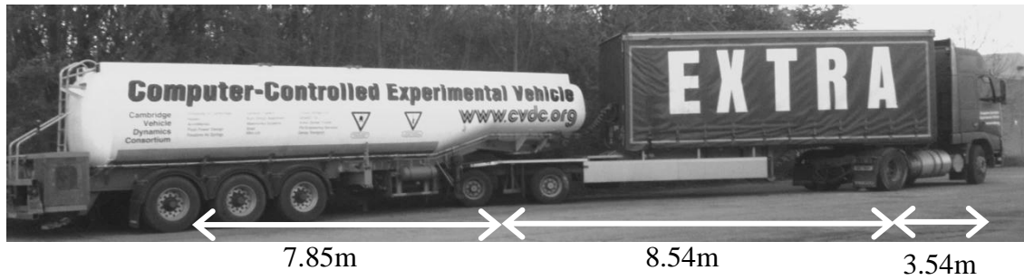
Figure 1: B-double test vehicle: The Denby ‘Extra’ Eco-Link B-trailer was loaned by Denby transport. The other vehicle units are part of the CVDC test vehicle fleet. Distances shown between the front axle and the hitch point for the tractor unit, hitch to hitch for the B-trailer and hitch to equivalent rear axle for the tanker.
