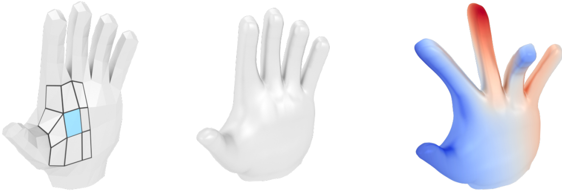
Figure 1: Isogeometric analysis using manifold-based smooth surfaces. The smooth surface in the middle is described by the control mesh on the left and the corresponding manifold basis functions. The deflected geometry on the right is the result of a finite element thin-shell computation with manifold basis functions.
