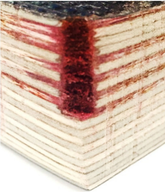
Figure 2. Diffusion of red dye outward from a central hole indicates that moisture has a tendency to travel parallel to the grain through vessels in individual veneers.
