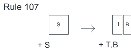
Figure 10.81: Rule for separation bath and toilet.
